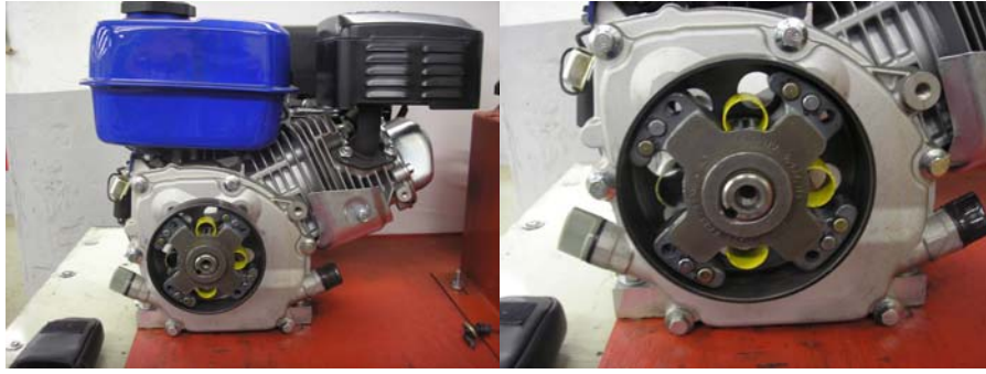
Above: Leading Shoe – Inboard Mounted (Sprocket toward Engine) (Cover Removed for Clarity)
