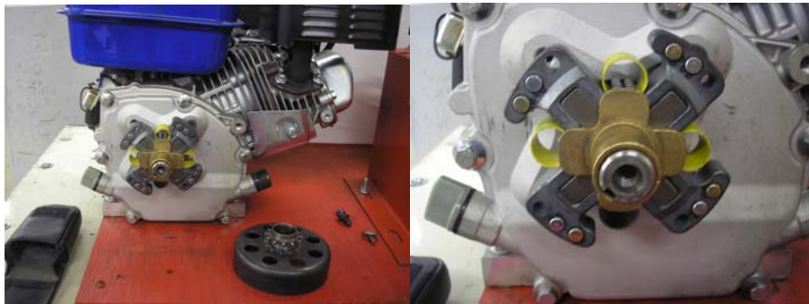
Above: Leading Shoe – Outboard Mounted (Sprocket away from Engine) (Drum Removed for Clarity)
