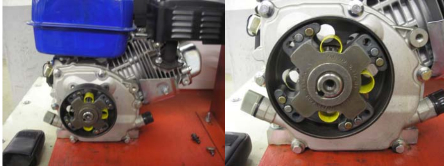
Above: Trailing Shoe - Inboard Mounted (Sprocket toward Engine) (Cover Removed for Clarity)
