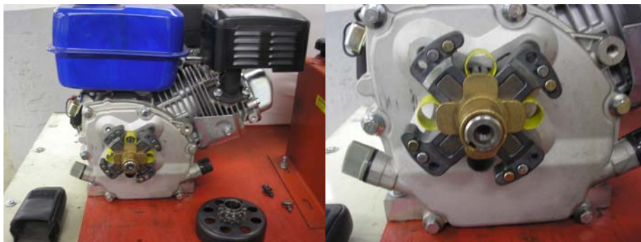
Above: Trailing Shoe – Outboard Mounted (Sprocket away from Engine) (Drum Removed for Clarity)
